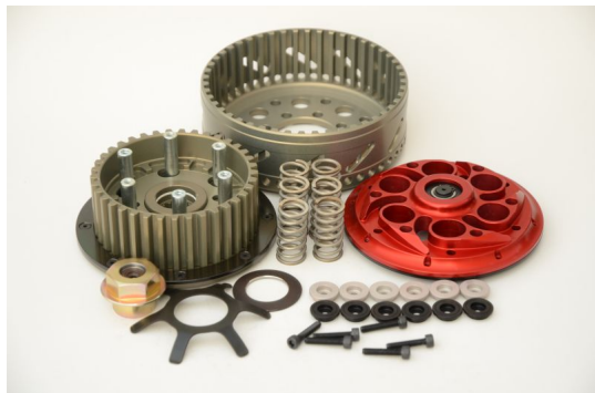
Slipper clutch for motorbike DUCATI 848 (48T) with Performance dry clutch kit
